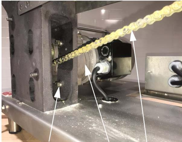
Motor Mounting Bolt      Gear Motor      Drive Chain
