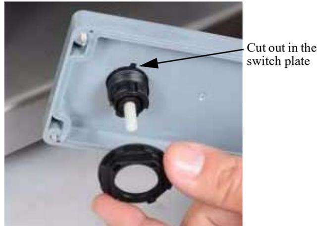
**Step 7:** Install the locking ring and tighten.
