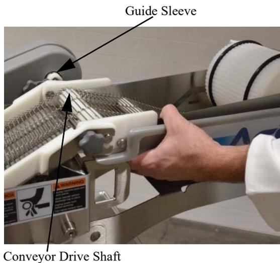
**Step 3:** Remove the batter conveyor tank assembly.
