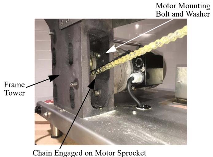
**Step 14:** Adjust the drive chain tension by allowing the weight of the motor to tension the drive chain. To avoid over tensioning the drive chain, make sure the drive chain has 3/4" slack as shown. Tighten the (4) motor mounting bolts.
