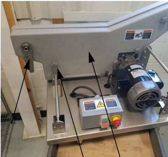
Locking Latch      Knobs      Drive Guard Cover
