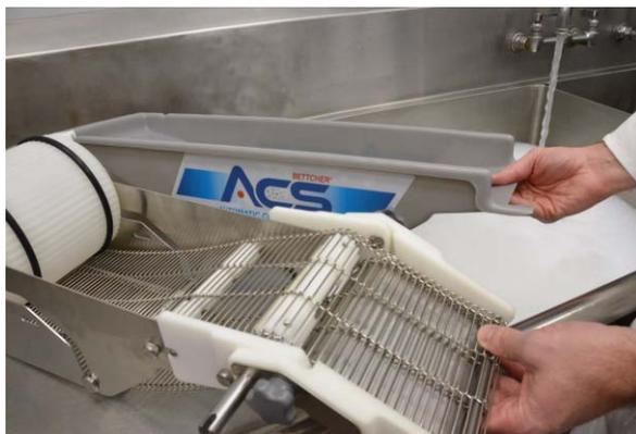
**Step 7:** After the components are dry, place the batter conveyor assembly into the batter tank.
