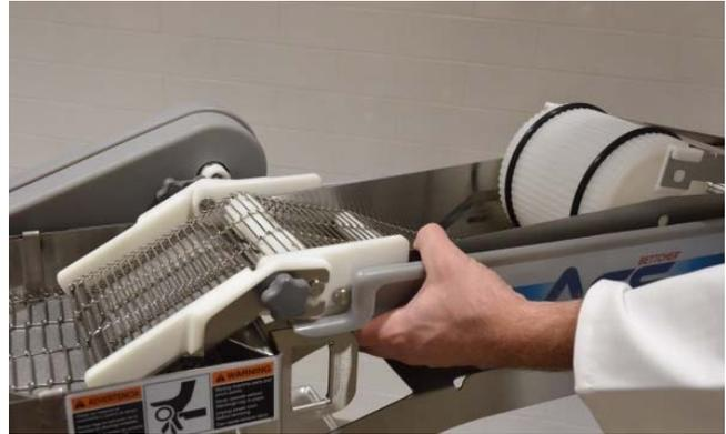
**Step 12:** Align the conveyor driven shaft with the bearing guide sleeve on the frame assembly.
