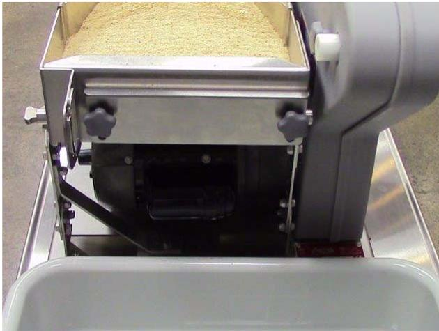
**Step 2:** Loosen knobs and open discharge cover.
