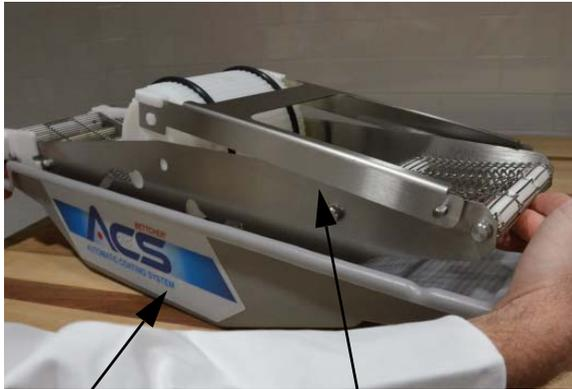
Batter Tank                      Batter Conveyor Assembly
