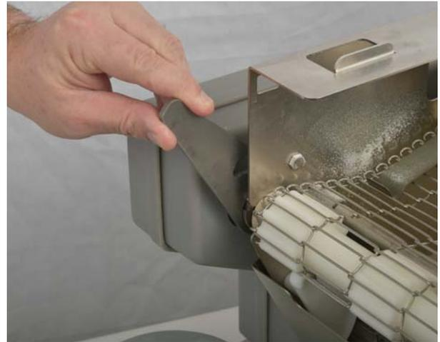
**Step 7:** Support breader at the front with left hand on the sprocket and right hand at the rear. (Place thumb through the handle with fingers supporting bottom pan.) Remove.
