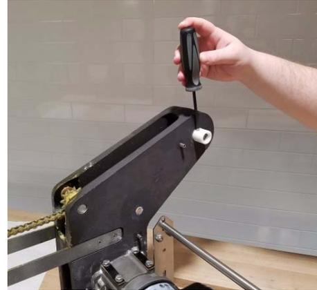
**Step 13:** Adjust the drive chain tension by allowing the weight of the motor to tension the drive chain. To avoid over tensioning the drive chain, make sure the drive chain has 3/4" slack as shown. Tighten the 4 motor mounting bolts.
