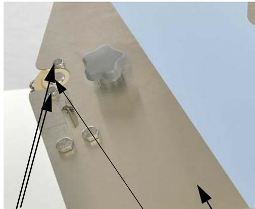
Retaining Screws    Bearing    Side Rail
