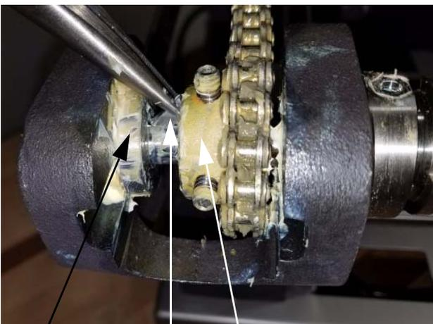
Spacer Ring    Sprocket Key
