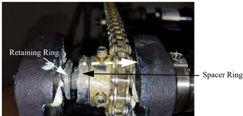
**Step 8:** Slide the drive shaft out of the bearing assemblies. While sliding the old shaft out, be certain to hold onto the loose components on the shaft (thrust bearings, thrust washer, spacer ring and drive sprocket) to prevent loss.
